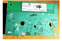
Note the corrosion on the circuit board contacts.
