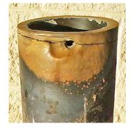
Nearly 2' of pipe was cut out of the line including the break and a valve was inserted in that space to
